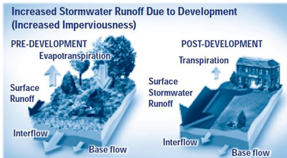
Figure 2. The impacts of development on runoff processes (Centre for Watershed Protection, 1999).
