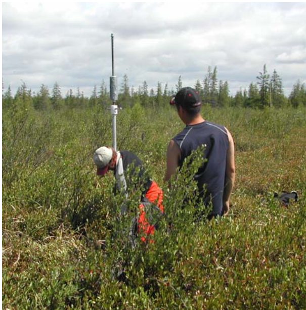
Fig. 5A. The core sampler is inserted into the peat
