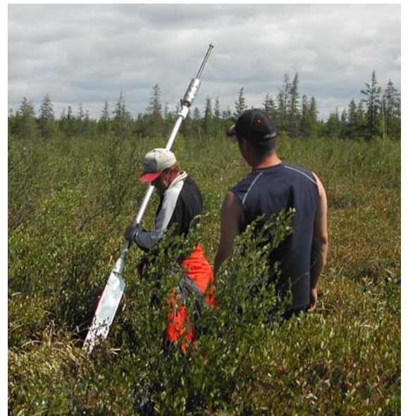
Fig. 5B. The core sampler is retrieved.
